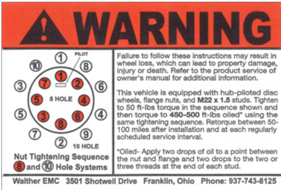
Figure 41 – Hub-Piloted Torque Sequence
