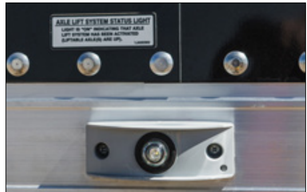
Figure 24 – Axle Lift System Decal and Light
