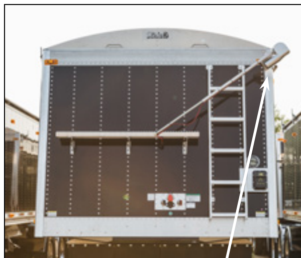
Figure 23 – Electric Tarp Drive
