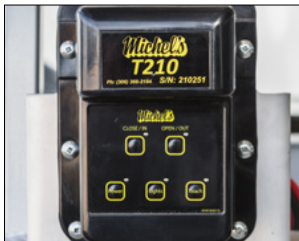
Figure 24 – Tarp Control Box
