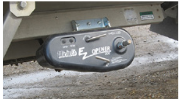
Figure 16 – Electric Chute Gate Drive
