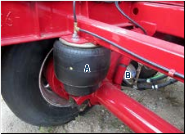
A – Air Bag B – Shock Absorber Figure 36 – Air Bags (Typical)
