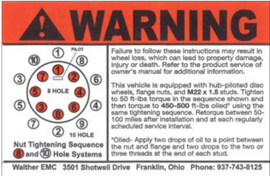
Figure 47 – Hub-Piloted Torque Sequence
