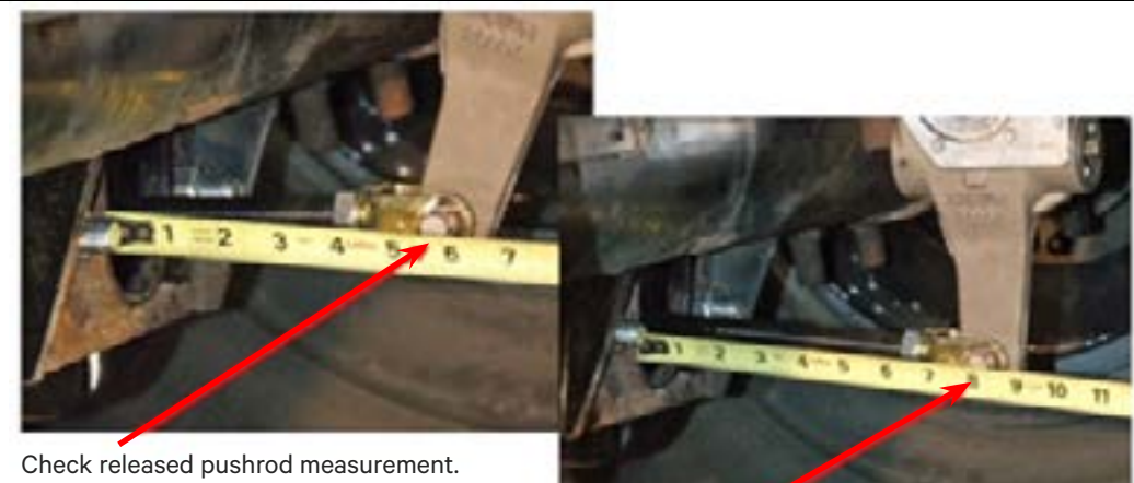
Figure 41 – Haldex Slack Travel Measurement
